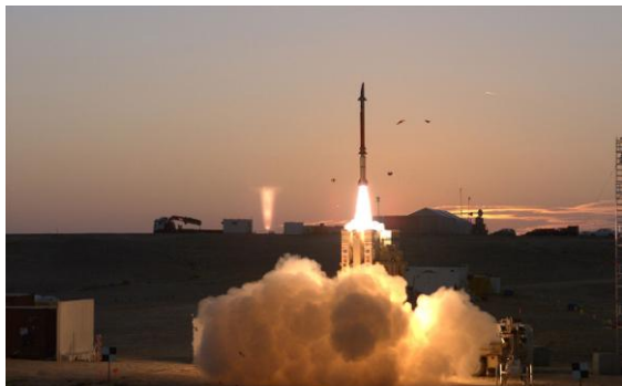
Stunner is a two-stage interceptor missile developed to intercept short-range ballistic missiles, large calibre rockets and cruise missiles and unmanned aircraft systems. Source: Army-technology.com
