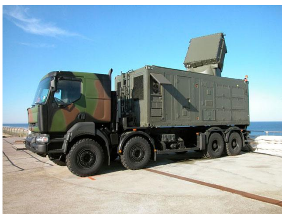
SAMP/T is a fully autonomous, self-propelled system with truck-mounted modules. Each system typically includes a Fire Control Unit, with a multi-function radar (MRI) and an Engagement Module (ME), and launching elements, with up to 6 vertical launch platforms (MLT) using Aster 30 missiles. Source: Eurosam.com
