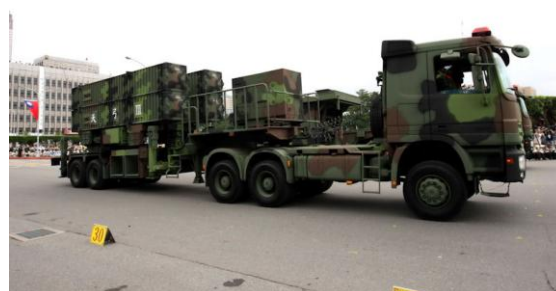
The Tien Kung III (Sky Bow III) surface-to-air missile system was developed by the Chungshan Institute of Science and Technology to counter tactical ballistic missiles. Source: GlobalSecurity.org
